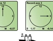
3. Turn shafts with measuring units to position 9, 12 and 3 o'clock.
