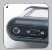
Countersunk connectors, well protected against external damage.
