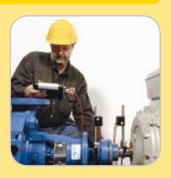
display through the entire measurement procedure. Even though the technology inside is rather advanced, the measurement principle is straightforward. It is based on the "reverse indicator method" with two laser/measuring units mounted on each side of the coupling.
