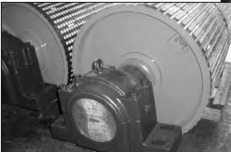
Engineering Drum Pulley assembly with keyless locking device. Ceramic Lagging.
